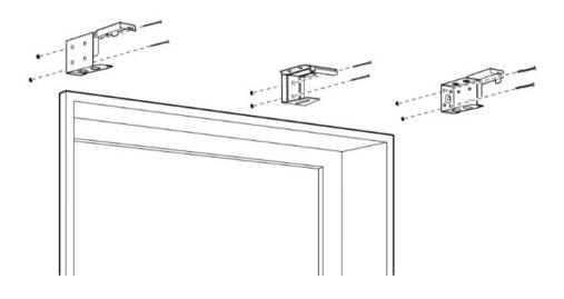
If using a center bracket, screw the widest end into the top of the frame.
