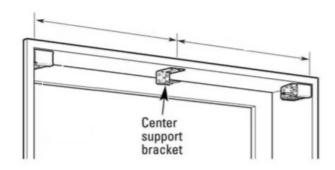
• If using a center bracket, screw the widest end into the top of the frame like a U shape turned on its side with the open section facing you.
